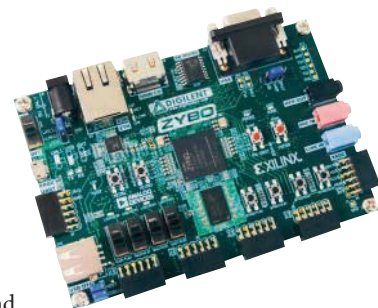
3. Digilent's ZYBO (Zynq Board) has 512 Mbytes of RAM and six Pmod connectors.
