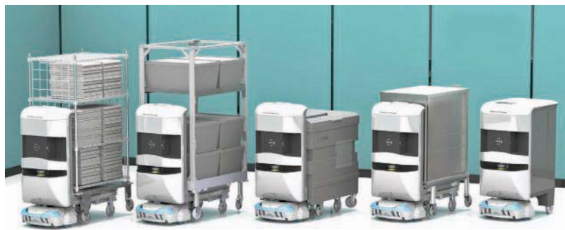
5. Aethon's Tug pulls a trailer that can deliver drugs from the pharmacy or lunch from the cafeteria throughout a hospital.
