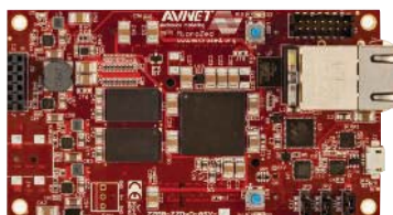
2. Avnet's MicroZed exposes more than 100 I/O ports using two connectors on the bottom.
