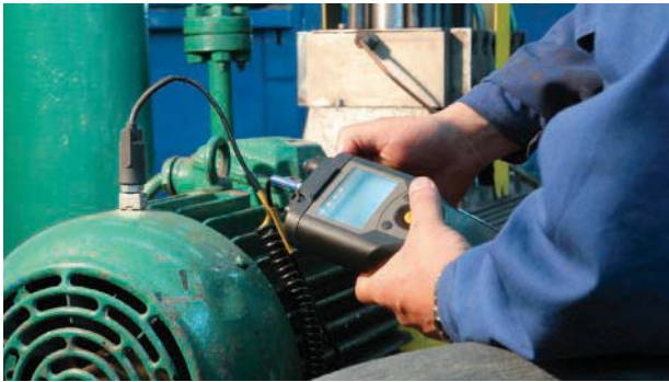
2. Existing manual probe methods for equipment vibration shift monitoring lack repeatability and reliability.
