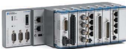
1. National Instruments' cRIO-9068 is based on Xilinx's Zynq-7000. It runs Linux and LabVIEW applications.
