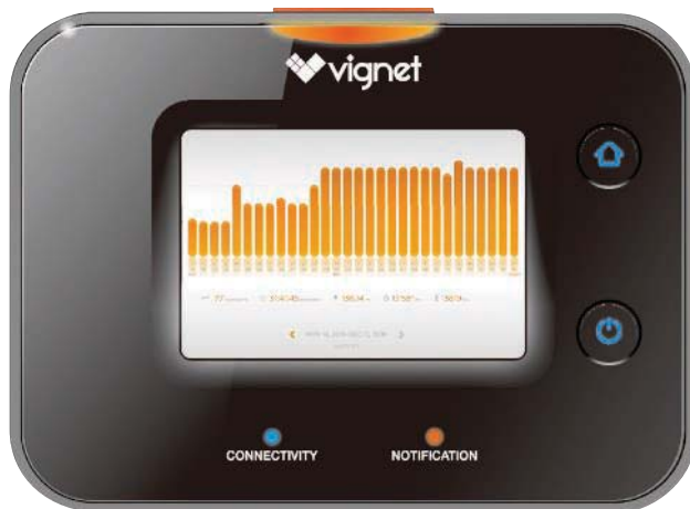
3. The Vignet hub collects patient monitoring data with Bluetooth or Wi-Fi and then transmits it over the cellular network using Gemalto's Cinterion embedded cellular transceiver.
